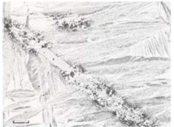
Figure 1746. Tishomingo. A daubreelite-troilite aggregate in martensite. The troilite is shock-melted while the daubreelite (D) has survived intact. Etched. Scale bar 100 \mu .
