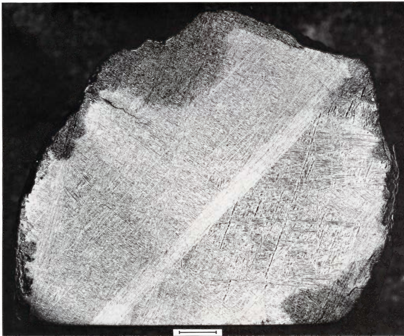
Figure 1742. Tishomingo. A part slice showing the anomalous, coarse martensitic structure. An austenite twin crosses the entire section. Terrestrial corrosion penetrates irregularly from the surface (black patches). Etched. Scale bar approximately 4 mm. S.I. neg. 1470C.
