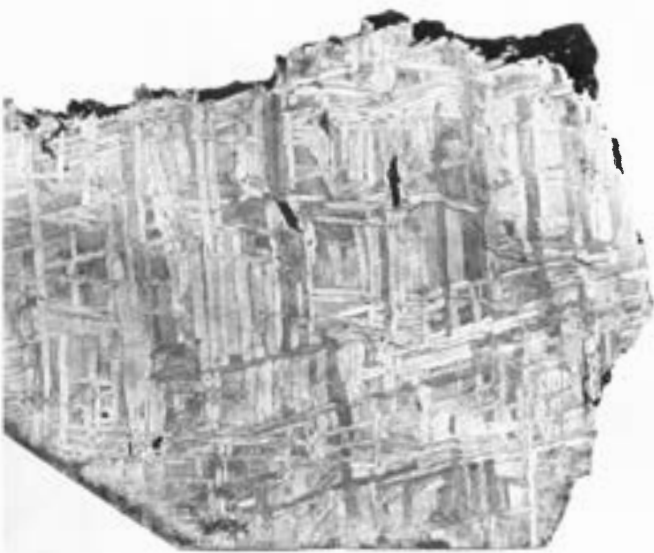
Figure 1703. Tamarugal (Copenhagen no. 1908, 80). A medium octahedrite that is transitional between group IIIA and IIIB. Deformed Widmanstätten pattern and troilite nodules (black). Etched. Scale bar 20 mm.
