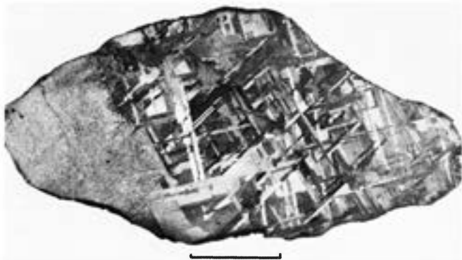
Figure 1001. Kingston (U.S.N.M. no. 539). An anomalous medium octahedrite. The characteristic matte structure at one end appears to be due to artificial reheating. Deep-etched. Scale bar 30 mm. S.I. neg. 33199A.
