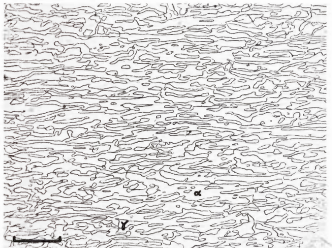
Figure 1013. Kokomo (Copenhagen no. 1876, 2245). The \alpha + \gamma matrix displays oriented intergrowth. There are indistinct sub-boundaries in the \alpha -phase. Etched. Scale bar 30\ \mu .
